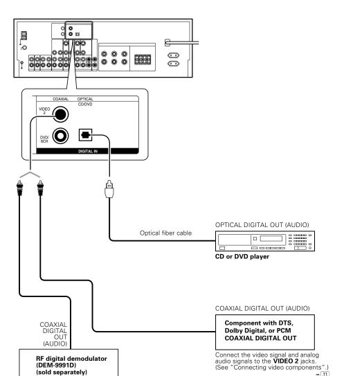
To connect an LD player with a DIGITAL RF OUT, connect the LD player to the KENWOOD RF digital demodulator (DEM-9991D). Next, connect the DIGITAL OUT jacks of the demodulator to the DIGITAL IN jacks of the receiver. Connect the video signal and analog audio signals to the VIDEO 2 jacks. (See "Connecting video components".)
